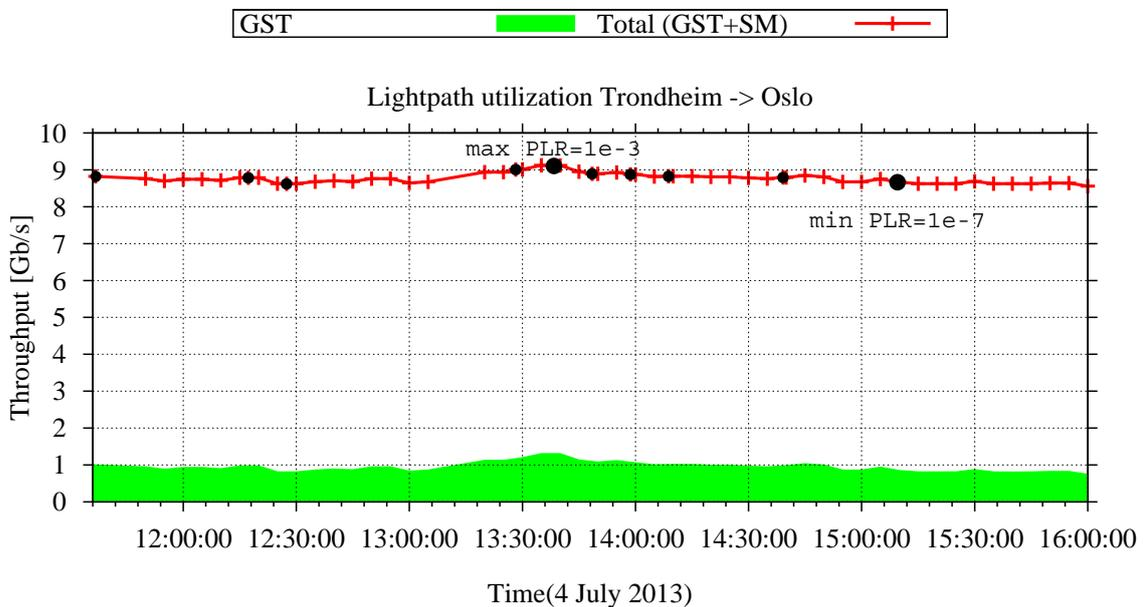
Figure 4. Average link throughput as a function of time of day. The production traffic is carried as GST depicted with the filled lower curve (green). The total throughput with added SM traffic is depicted by the curve (red) to an average of 88% of the capacity. The points are marking the observation of SM losses. GST statistics are collected by the Fusion nodes with 5 min sampling and for SM by the Spirent traffic generator/analyzer with 10 min sampling.
