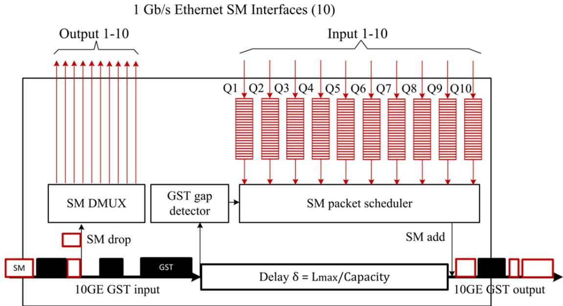
Figure 1 Schematic diagram of the unidirectional (left to right) transport through the fusion hybrid node with ten 1 Gb/s Ethernet interface for local add/drop and one 10Gb/s Ethernet wavelength. The gigabit Ethernet interfaces are depicted logically divided into input and output interfaces to better illustrate the de-multiplexing of SM traffic when entering the node and the scheduling of input traffic in available gaps in the output wavelength.
