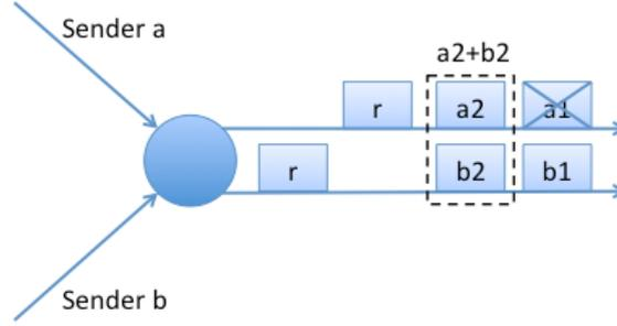
Figure 2: NLPRS extended with network coding. Two packet sets from different ingress nodes collide at an OPS core node.
