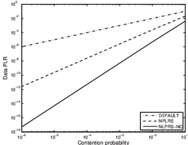
Figure 3: Packet loss rates using the analytical model,  $m = 5$  and  $r = 1$ .
