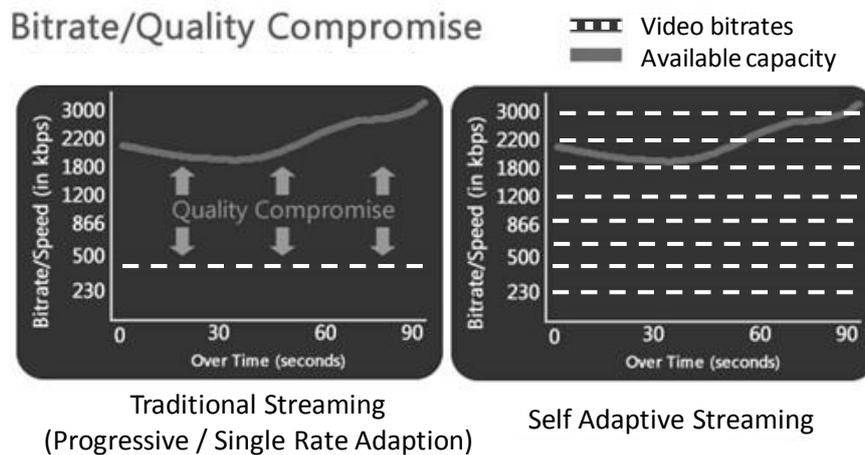
Figure 2 Traditional vs. Adaptive Streaming
