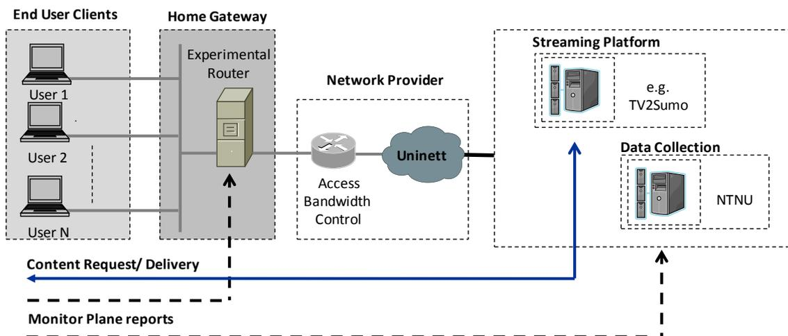
Figure 3 Monitor Plane component testbed
