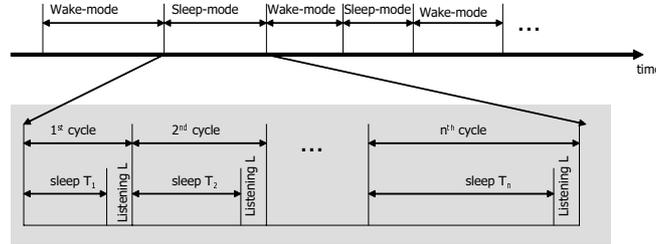
Figure 1 Wake mode and sleep mode transition in the IEEE 802.16e
