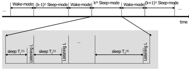
Figure 2 Enhanced energy management mechanism in IEEE 802.16e
