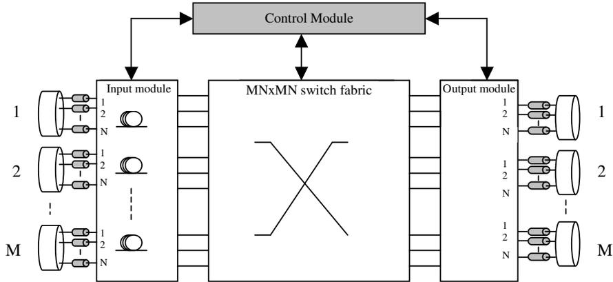
Figure 1: Overview of an optical packet switch.
