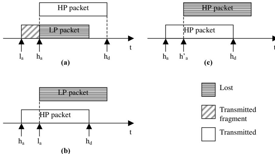
Figure 4: The different preemption scenarios in the PDP
