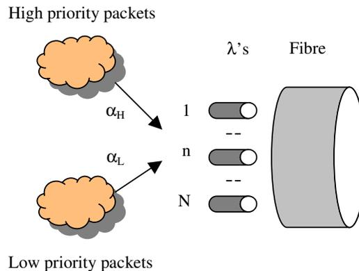
Figure 2: Traffic model of an output fibre
